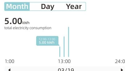
The switch can monitor the current, voltage and power of the load equipment in real time, and can also record the power consumption of the year, month, day, hour and different time periods, helping users check the power consumption of load equipment more clearly. Setting the switch status of the equipment in different scenarios, and remotely monitor the real-time situation of the load electrical appliances.
