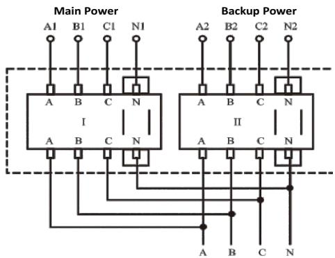
Position “II”; Connect main power again, the switch shall be at Position “I”.
